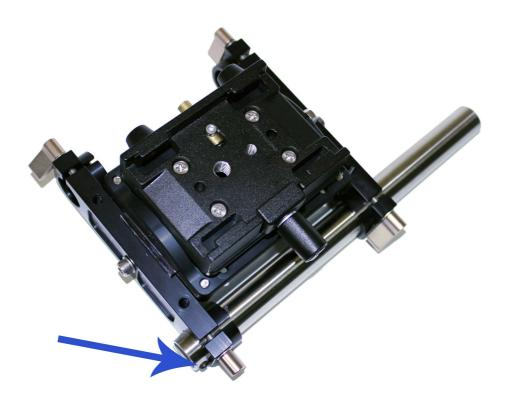
Now slide this assembly on to the short rod attached to the front square rail so that the both short stainless steel rods now go into the square rail. Secure the remaining two gold locking tabs on the lower platform assembly using finger pressure. All four gold tabs should be finger tight.
