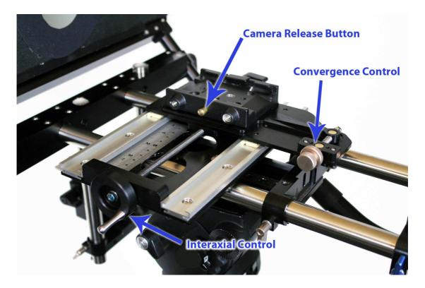
The cameras/lenses should be centered over the mounting plates for maximum stability. The entire camera platform can be slid along the rod by slackening the gold tabs. Once you have positioned the cameras and camera platforms tighten all the gold tabs, 6 on the top platform and 4 on the lower.
