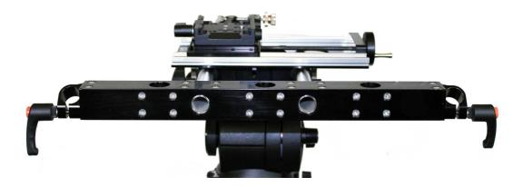
The rods should be flush with the front of the square front rail. Secure by tightening (clockwise) the two allen (hex) head bolts recessed into the underside of the rail. Do not over tighten, use a short allen key and hand pressure only. Check the square rail assembly is firmly attached to the horizontal rails before proceeding to the next step.
