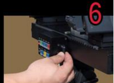
6 Connect the LANC cables and power cable to the mount control
