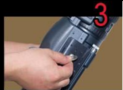
3 Attach the shoe to the camera
