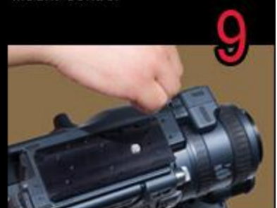
9 If the balance is not right, adjust the height of the shoe
