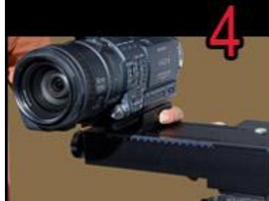
4 Insert and tighten the camera in the mount block
