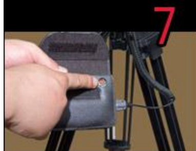
7 Supply power to the mount by pushing the power button at the battery
