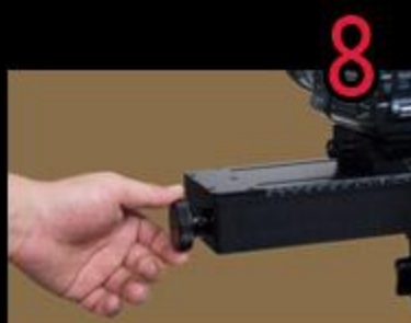
8 Adjust distance and angles of the two cameras
